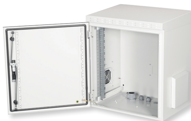
3-point locking system on the front door Base plate with cable feed Roof with cut-outs for ventilation
