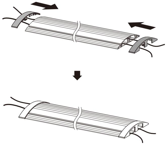
Re-attach the plastic end caps on each side of the ducting.
