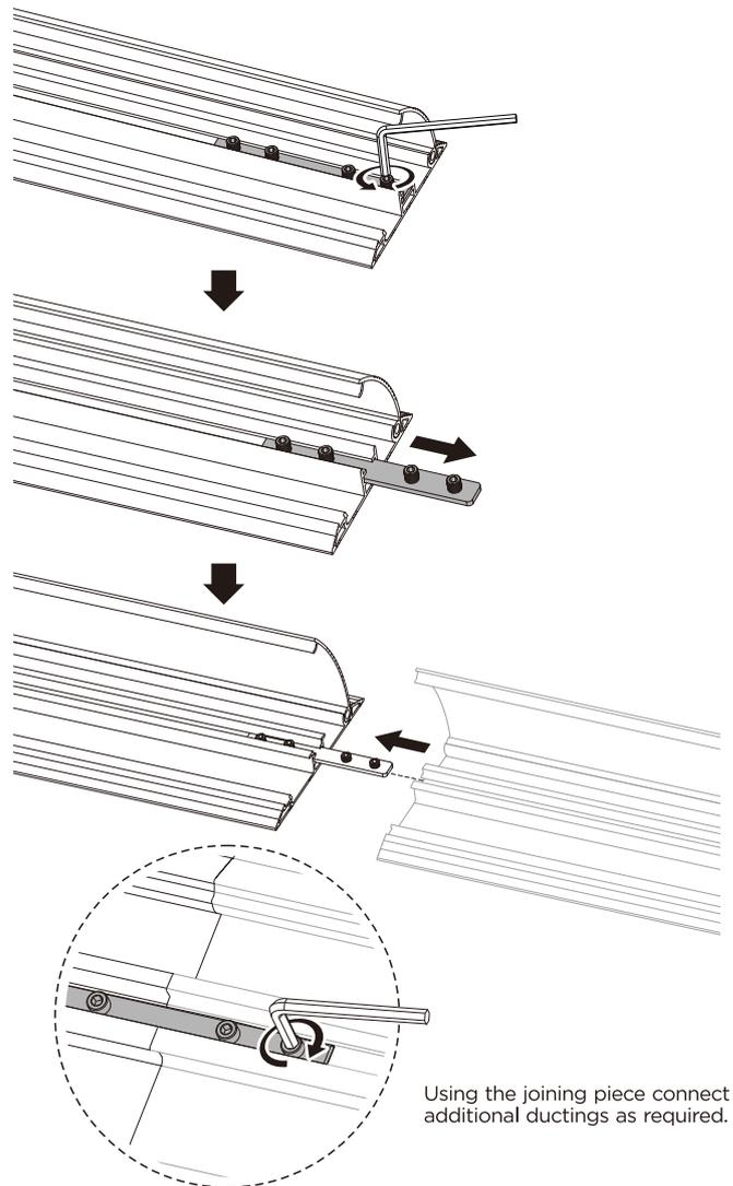
Using the joining piece connect additional ductings as required.
