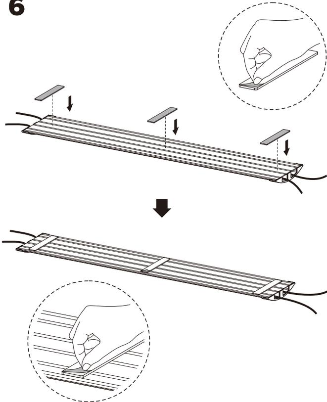
To prevent the ducting from moving, attach double-sided tape as required.
