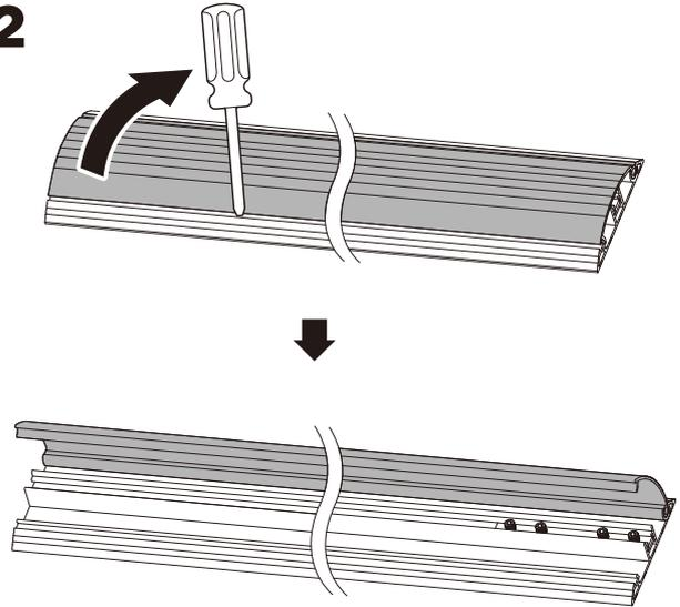
Using a flat tipped screwdriver gently pry open the cover as shown.
