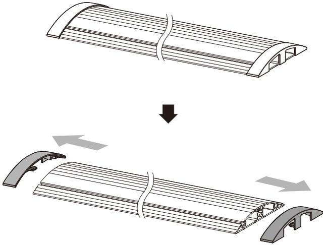
Remove the plastic end caps on each side of the ducting.
