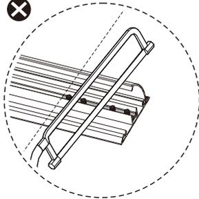
Using a hacksaw cut the ducting to desired length
