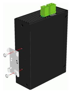
2. Attach the bracket to the lower edge of the DIN rail and push the unit upwards a little bit until the bracket can clamp on the upper edge of the DIN rail.
