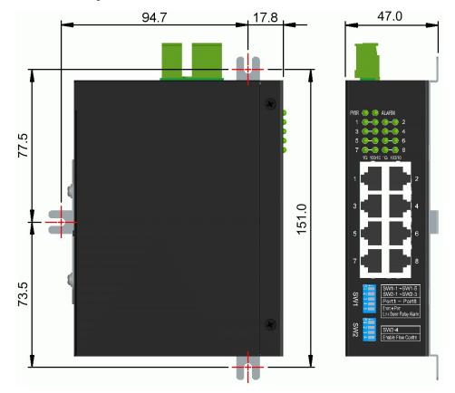
3. Screw the switch unit on a panel. The locations for screws are shown below:
