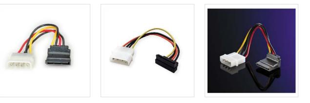
Adapter cable for converting the 4-pin HDD interface to the SATA power connector; 4-pin HDD plug to 15-pin SATA power connector; angled (90°); length: 0.1 m
