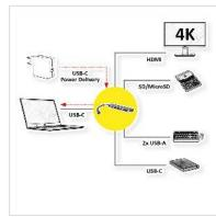
The USB Type C Docking Station provides your MacBook, Ultrabook, Notebook or Laptop with 1x 4K HDMI, 1x USB 3.0 Type A, 1x USB 2.0 Type A, 1x USB 2.0 Type C, 1x SD/Micro SD, 1x USB Type C PD (Power Delivery).
