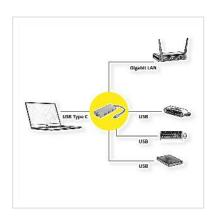
With this converter you can connect your MacBook, Ultrabook, Laptop/Notebook or PC with USB Type C interface to a Gigabit Ethernet network and up to three USB 3.0 / USB 3.2 Gen 1 Type A devices.
