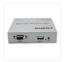
The KVM extension transmits HD audio and video signals as well as USB signals up to 20 km via a bidirectional fiber optic single-fiber cable. This allows a computer system to be controlled up to 20 km away via the remote console (HDMI 4K monitor, USB keyboard and USB mouse).
