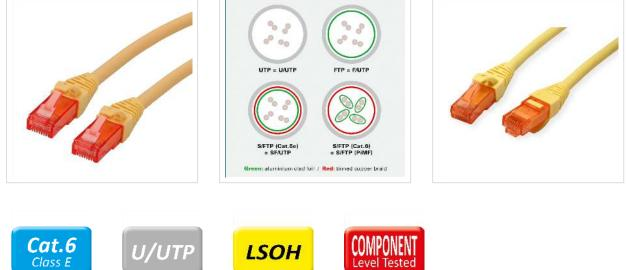
Patch cable for networking connections between devices. Prepared unshielded Twisted Pair cable with RJ-45 connectors on both ends. Durable due to moulded kink protection. Flexible cable, suitable for narrow bending. High quality plugs with gold plated contacts. Contact settings 1:1, in accordance with the EIA/TIA 568 standard. Construction: 4-pair stranded copper wire. Halogen-free, flame retardant, low smoke.
