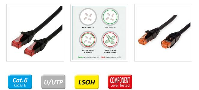
Patch cable for networking connections between devices. Prepared unshielded Twisted Pair cable with RJ-45 connectors on both ends. Durable due to moulded kink protection. Flexible cable, suitable for narrow bending. High quality plugs with gold plated contacts. Contact settings 1:1, in accordance with the EIA/TIA 568 standard. Construction: 4-pair stranded copper wire. Halogen-free, flame retardant, low smoke.
