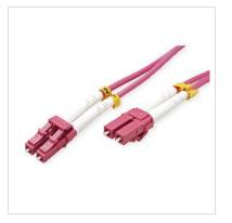
OM4 fiber for existing 1 and 10 Gbit/s applications as well as future 40 and 100 Gbit/s systems. Allows extended reach upwards of 550 meters at 10 Gbit/s for ultra long building backbones and medium length campus backbones. With an laser bandwidth of 4700 MHz-km (more than double the IEEE requirement for 10 Gbit/s 300 meter support), the OM4 fiber is also especially well suited for shorter reach in data centers and high performance computing applications.
